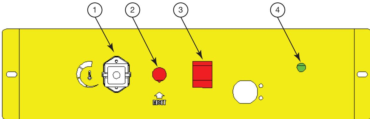
The heater is also equipped with an air pressure switch that controls the airflow pressure and locks the heater out in the event of unit overheating. If this occurs, detect and eliminate the cause of overheating before using the heater again. Have the heater inspected by a qualified technician if required. See point above for resetting.
