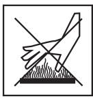
Serious injury may occur from touching the electrical motor. This area can remain hot for some time after the Biological Discharge System is shutdown. Never allow any part of your body to contact the electrical motor until cooled.
